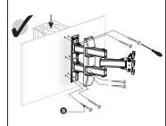
Using the provided self taping screws (B) type. Holding the TV mount starting in the one corner, screw the provided screws (B) into a wooden joist fixing the opposite corners, until the mount is secure onto the wall. Ensure all are tight and secure.
