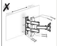
Ensure that the mount is fixed to a solid object and not into plasterboard on its own.
