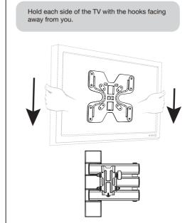
Slide the TV onto the bracket ensuring that the TV is centered onto the mount.
