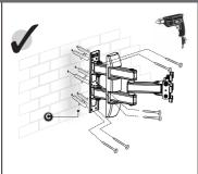
When selecting the position of the TV mount. ensuring that the mount will be mounted on to a flat surface and is level. Mark the wall where the fixing locations are. Drill the holes using a 10mm masonry bit. Using a hammer knock the the wall plugs (C) provided into the wall. Holding the TV mount start in the one corner screw the provided screws (B) into the wall fixing the opposite corners until the mount is secure onto the wall. Ensure all are tight and secure.
