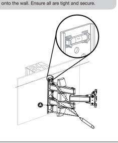
Using the provided self taping screws (B) type.
