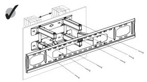
Using the provided self taping screws (C) type. Holding the TV mount starting in the one corner, screw the provided screws (C) into a wooden joist fixing the opposite corners, until the mount is secure onto the wall. Ensure all are tight and secure.
