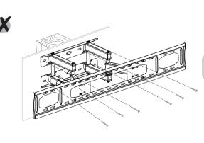
Ensure that the mount is fixed onto a solid surface and not directly onto plaster board.
