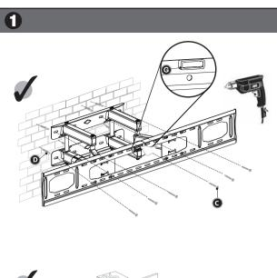
When selecting the position of the TV mount. ensuring that the mount will be mounted on to a flat surface and is level. Mark the wall where the fixing locations are. Drill the holes using a 10mm masonry bit. Using a hammer knock the the wall plugs (D) provided into the wall. Holding the TV mount start in the one corner screw the provided screws (C) into the wall fixing the opposite corners until the mount is secure onto the wall. Ensure all are tight and secure.
